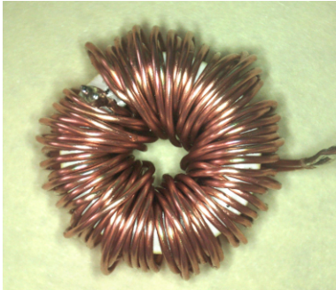
T13 56 \mu H double wire AWG25 on yellow/white toroid
